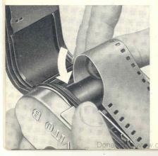
The narrow slit of the take-up spool must point upwards to take the beginning of the film. If necessary turn the take-up spool with the finger or by a few short movements of the rapid winder into the correct position. Then:
