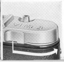
One full movement of the rapid winding lever, as far as it will go, tensions the shutter, and advances the film and film counter. The spring returns the lever to its original position each time.
